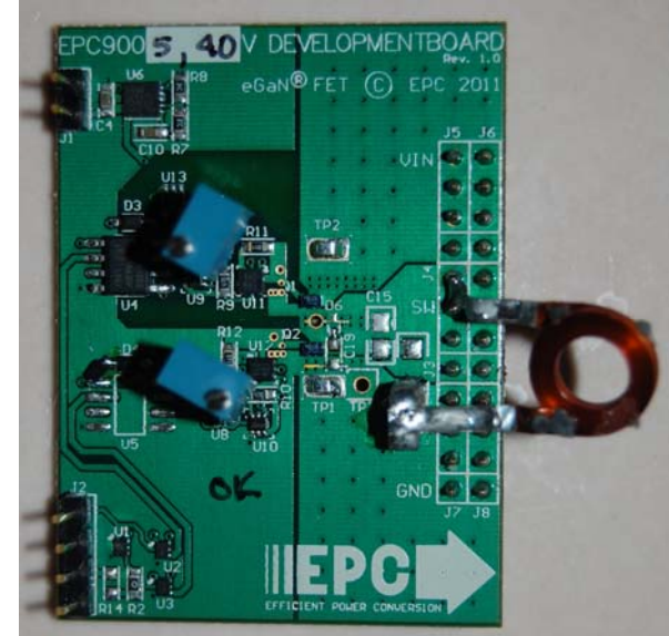
National eGaN Driver LM5113 on Bottom eGaN on Top side
