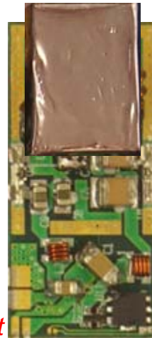
Test Board designed by David Lynn (BNL) Built by Chris Musso (NYU) with GLAST Silicon Strip Detector & Analog Readout
