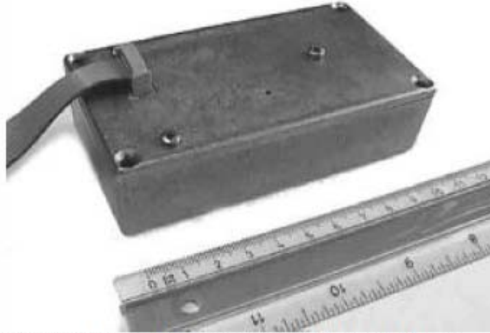
Figure 2 size of the converter (111x60x29mm, without connector and screws)
